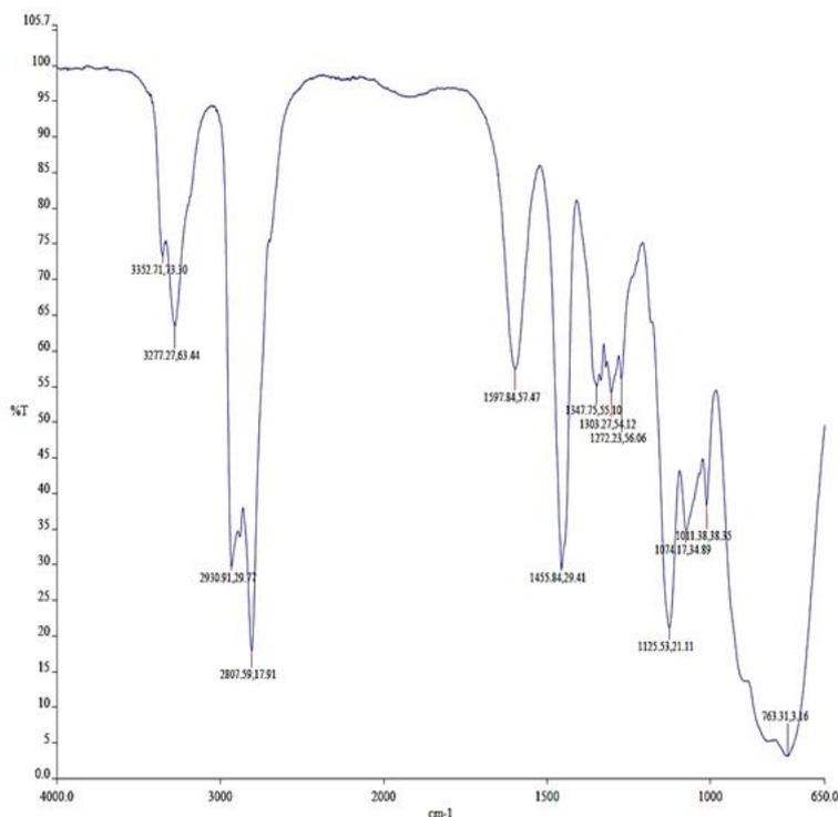
Fig. 6. IR spectrum of Triethylene tetramine
