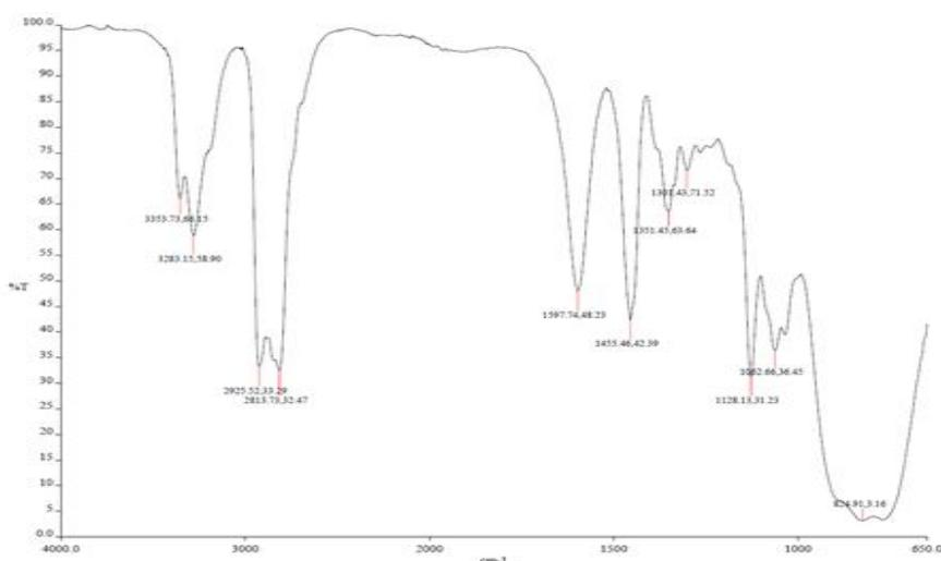
Fig. 3 IR spectrum of Waste PET with Diethylene triamine - After 8 days
