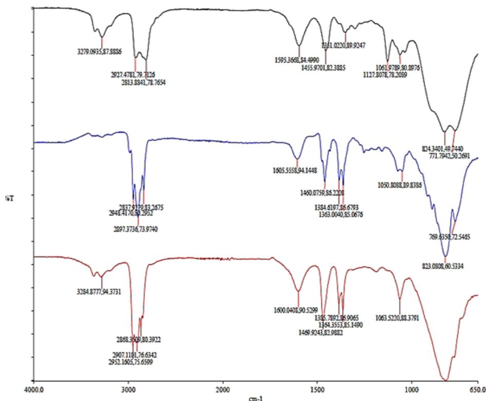
**Figure. 8 IR spectrum of waste PET & Diethylene triamine blend , waste PET & Isophoron diamine blend & waste PET & Trimethyl hexamethylene diamine blend after 7 days**
