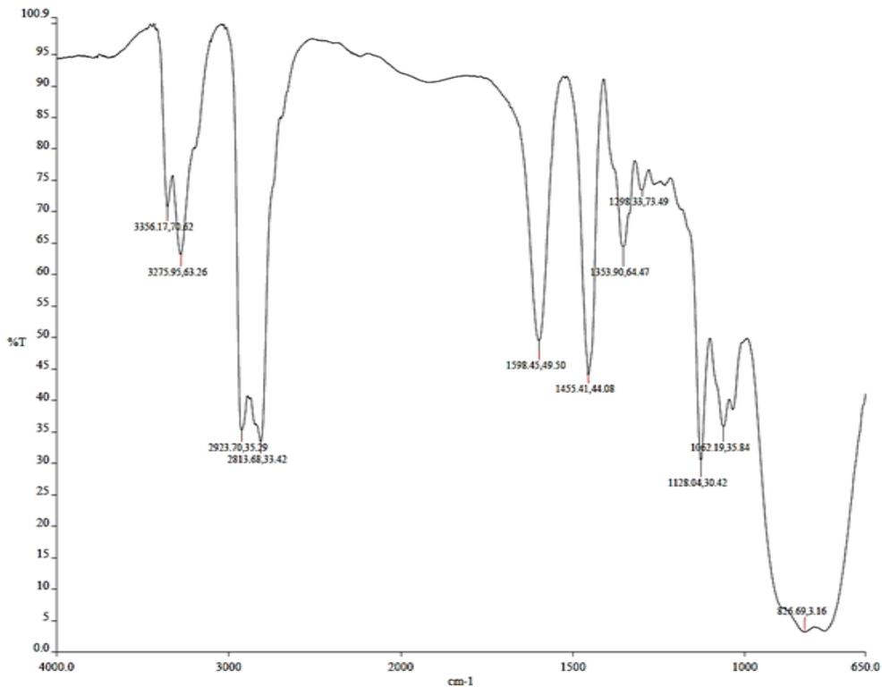
Fig. 5. IR spectrum of diethylene triamine
