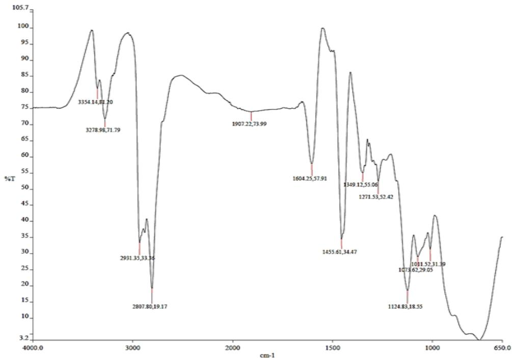
Fig. 4 IR spectrum of Waste PET with Triethylene tetramine - After 8 days
